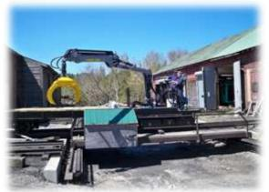
With his background designing weight-handling equipment for the U.S. Navy, LaPrade began in 2009 to sketch a custom flatbed car to hold a Kesla grapple loader, a Britton Stratton gas engine and Parker pump for the crane's onboard hydraulic power plant, plus a container cage for the collected rubble.
